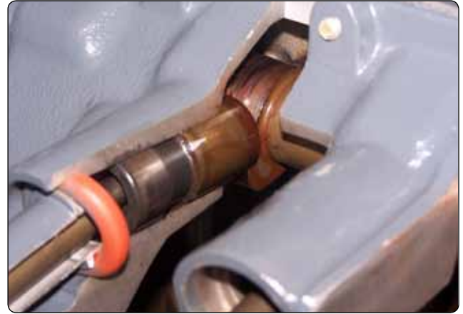
Figure 1-29. Cam load on lifter body.
