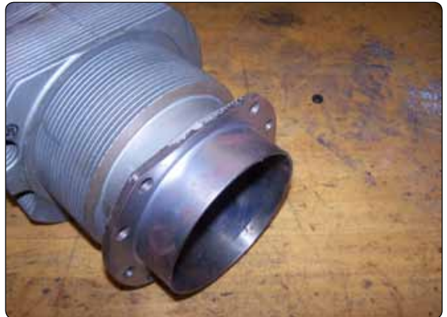
Figure 1-18. The aluminum head and steel barrel of a cylinder.
